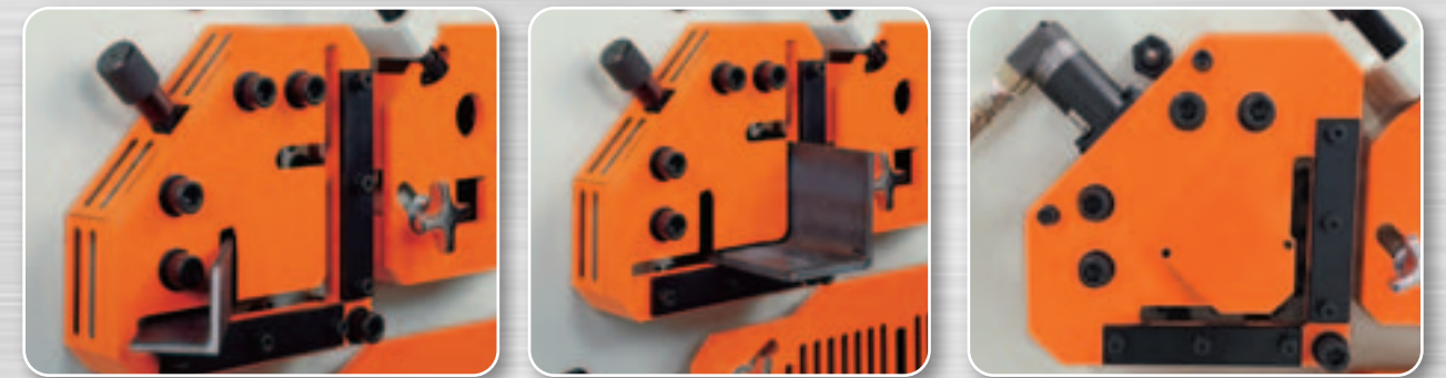
*Optional hydraulic hold-down for angle shear.
